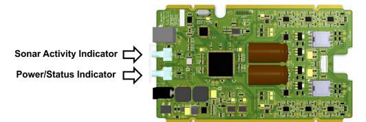
• Start the Scanline software or your application. When the software opens the data connection to the StarFish electronics and starts the sonar "pinging", the "Activity Indicator" will start to flash.
