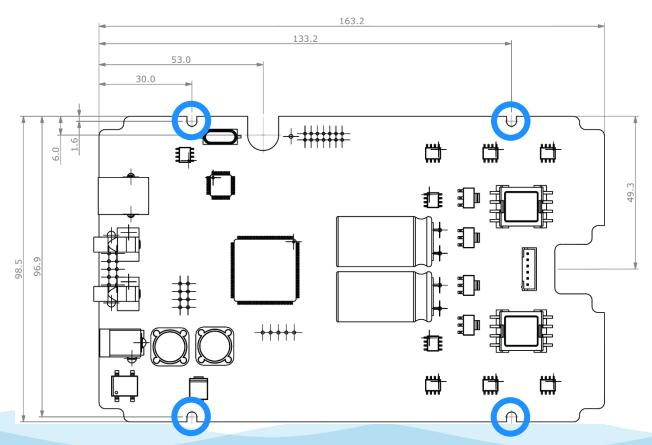
The should be stood off a base plate using spacers with a minimum height of 3mm.
