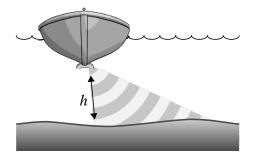
Therefore, the narrower the band of black is, the closer the sonar is to the seabed – and as the image is built up over time, if the sonar's altitude changes we actually start to see the profile of the seabed that the sonar has passed over.
