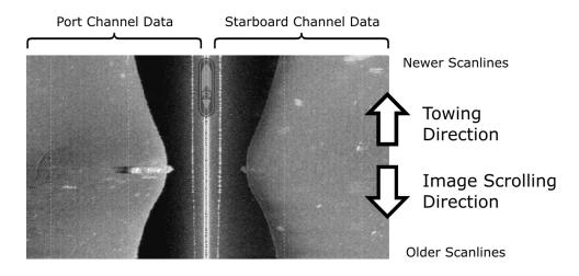
In this figure, both the port (left) and starboard (right) channels are operating at the same time. The sonar is positioned in the middle of the topmost line, and as the sonar is moved through the water the image will scroll away from it as more data is added.
